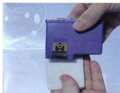
5. Take a piece of tissue and press it against the print head
